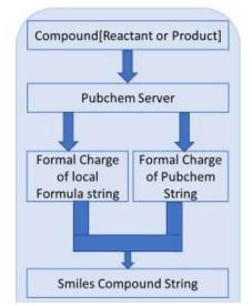
Diagram 2: The process flow diagram for Compound to Smiles String Conversion
