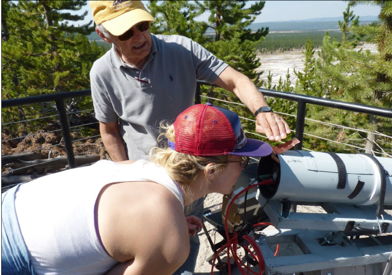
Fig. 12. VPL team member Kim Bott peers down the telescope of the Traveling Integrated Polarimetric Spectrograph for Yellowstone (TIPSY), built by Charles Telesco, University of Florida (grey shirt) to perform circular polarization measurements of microbes.
