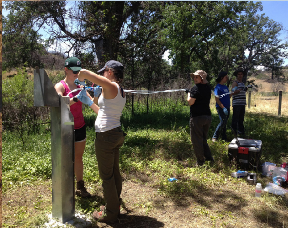
Fig. 1. RPL NAI team members at CROMO redeploying a pressure-temperature datalogger string into the CSW well to measure hydrogeological properties of the serpentinite subsurface. Credit: Matt Schrenk
