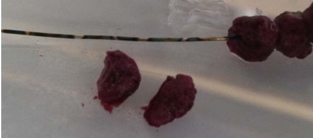
Removal of berry aggregates from the wire, revealing the black tarnish-marks left by sulfide precipitation.
