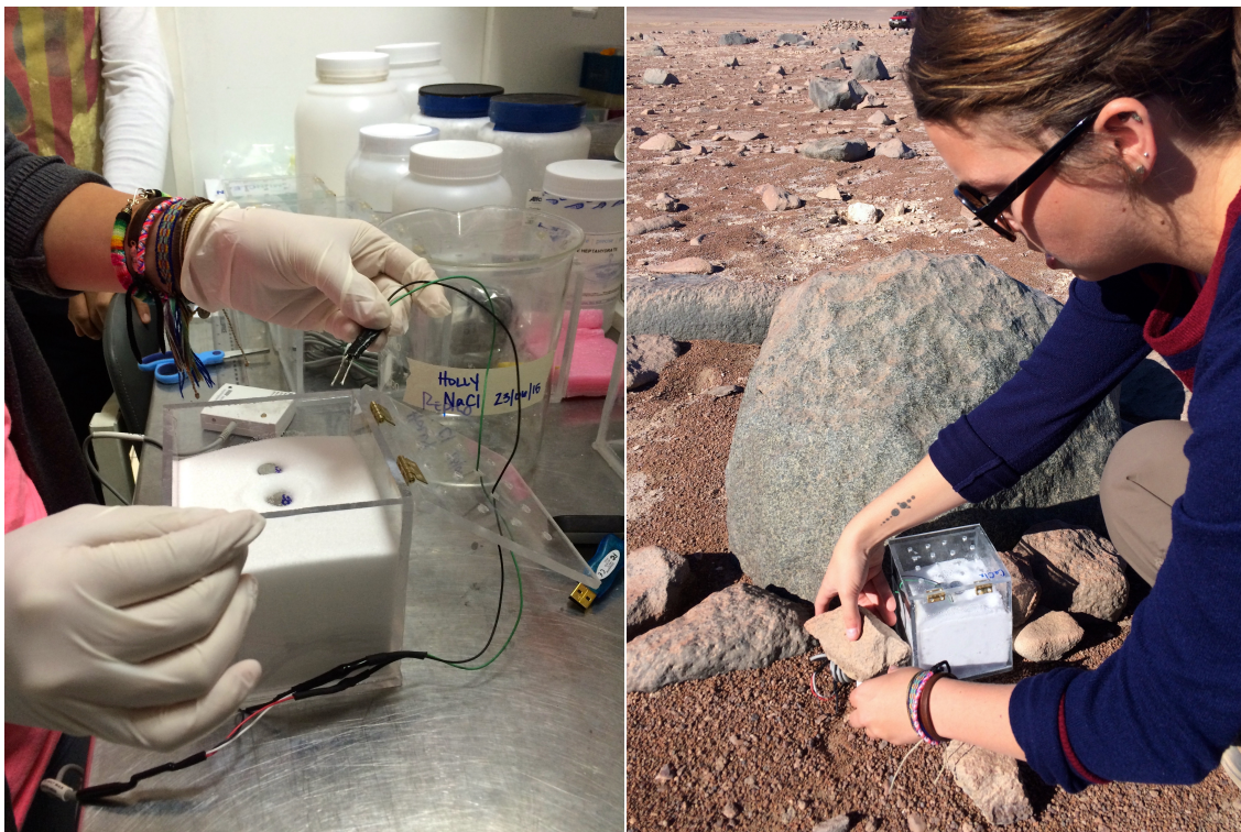
Figure 3 (Left): Installing iButtons and HOBO sensors while preparing samples in the laboratory. Figure 4 (Right): Using rocks to camouflage electronics while deploying sample in Yungay.
