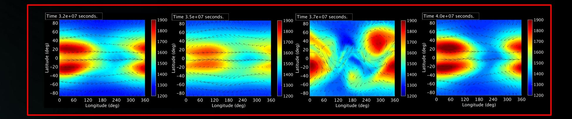
THOR is the first 3D atmospheric model that solves the deep-atmosphere non-hydrostatic Euler equations in an icosahedral grid dedicated to the study of planetary atmospheres.
