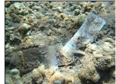
Figure 2. Artificial substrates. Microbial growth can be seen on copper (left) and stainless steel (right) pieces placed in Río Mesquites.
