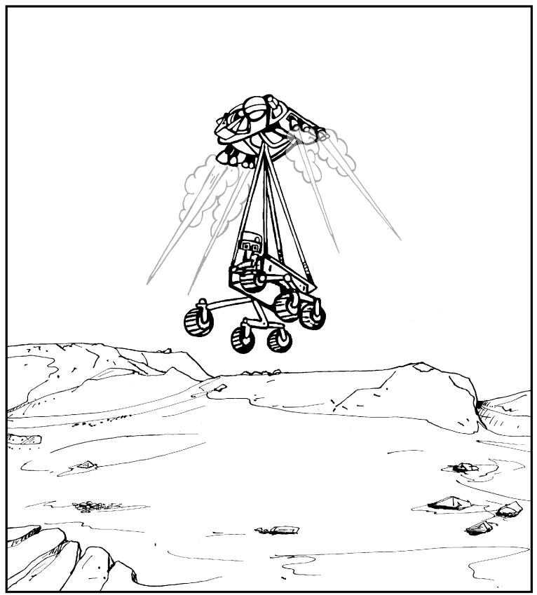
NASA's Perseverance rover is lowered to the surface of Mars using a 'sky crane.' This flying platform can gently place a rover down in a specific spot and then fly away. Sky crane technology has been used before by NASA, and successfully delivered the Curiosity rover to Mars in 2012.
