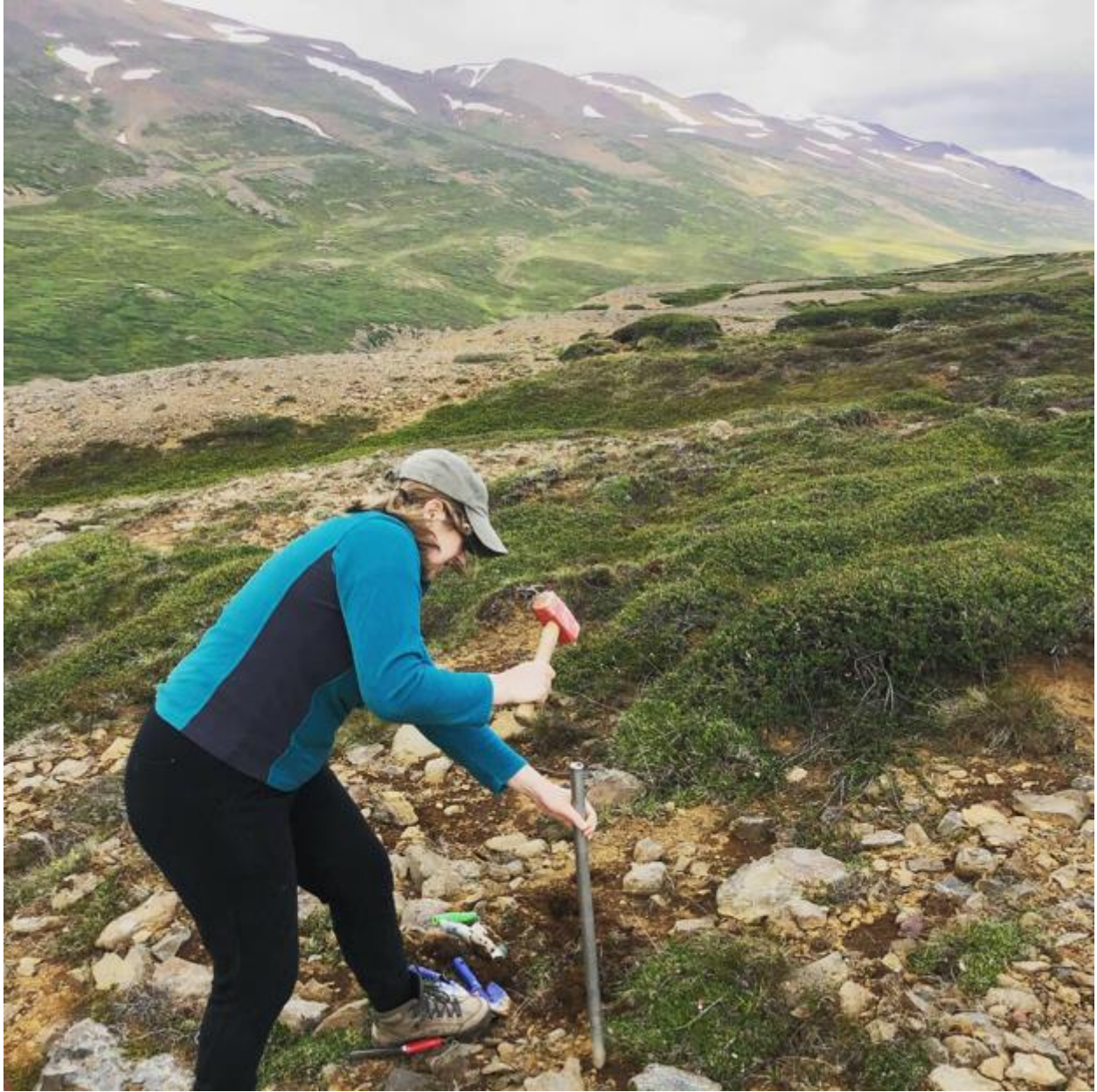
Figure 2: Metal cores don't work so well in very rocky soil and sediment, and they are hard to sterilize between uses! Photo credit: Carlie Novak
