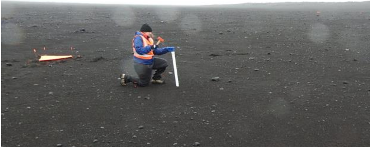
Figure 4: Taking a depth core at Dyngjusandur – we scrapped the metal sampling pipes, and decided to go with plastic pre-sterilized pipes instead. This worked much better! Photo credit: Erika Rader
