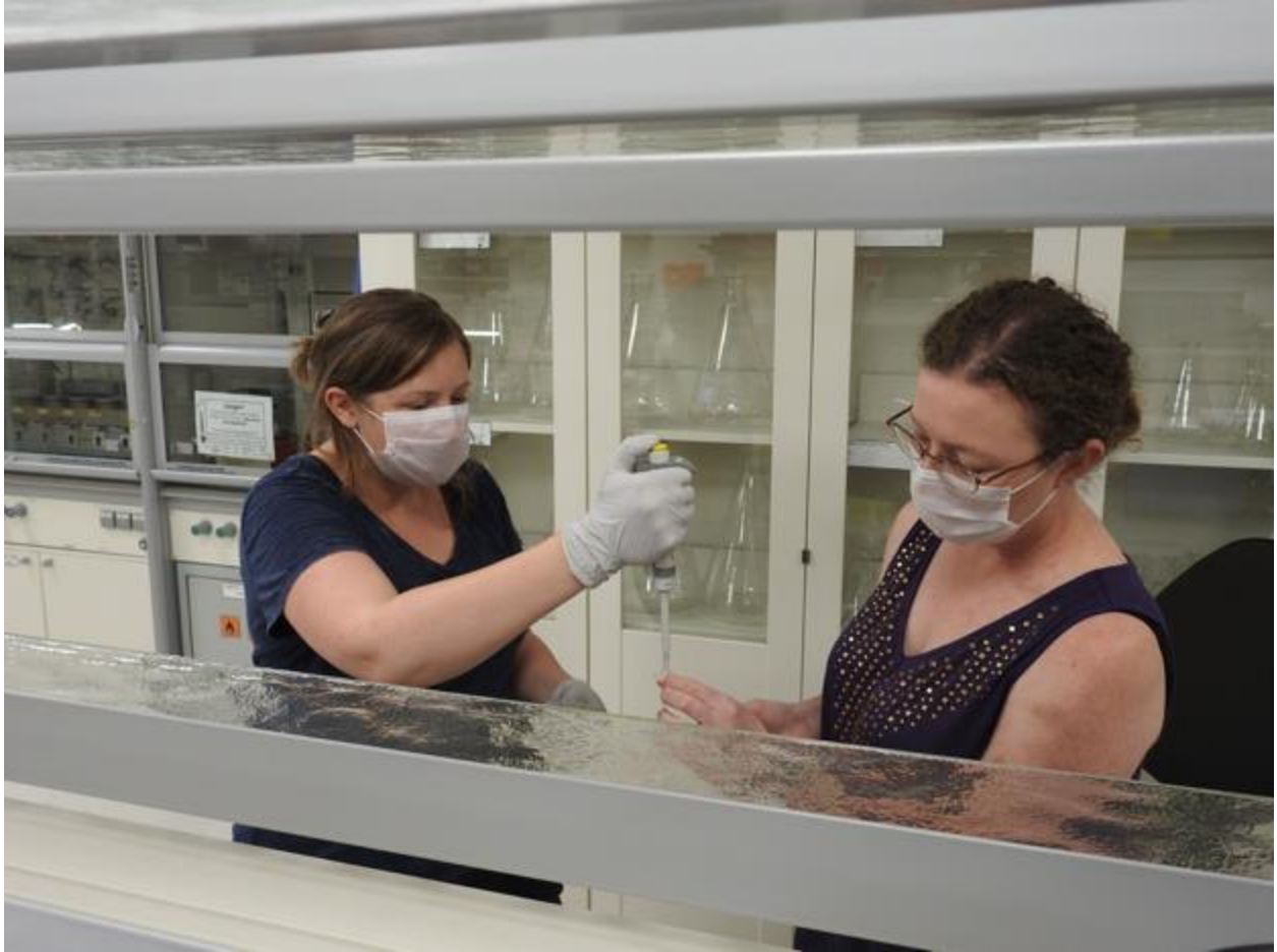
Figure 7: Performing ATP quantification assays at the University of Akureyri with Professor Amanda Stockton of Georgia Institute of Technology. The tubes that we use in the luminometer (which measures ATP activation of the enzyme luciferase) must be handled with bare hands rather than gloves, or they will build up an electrical charge and give inconsistent readings. Photo credit: Erika Rader
