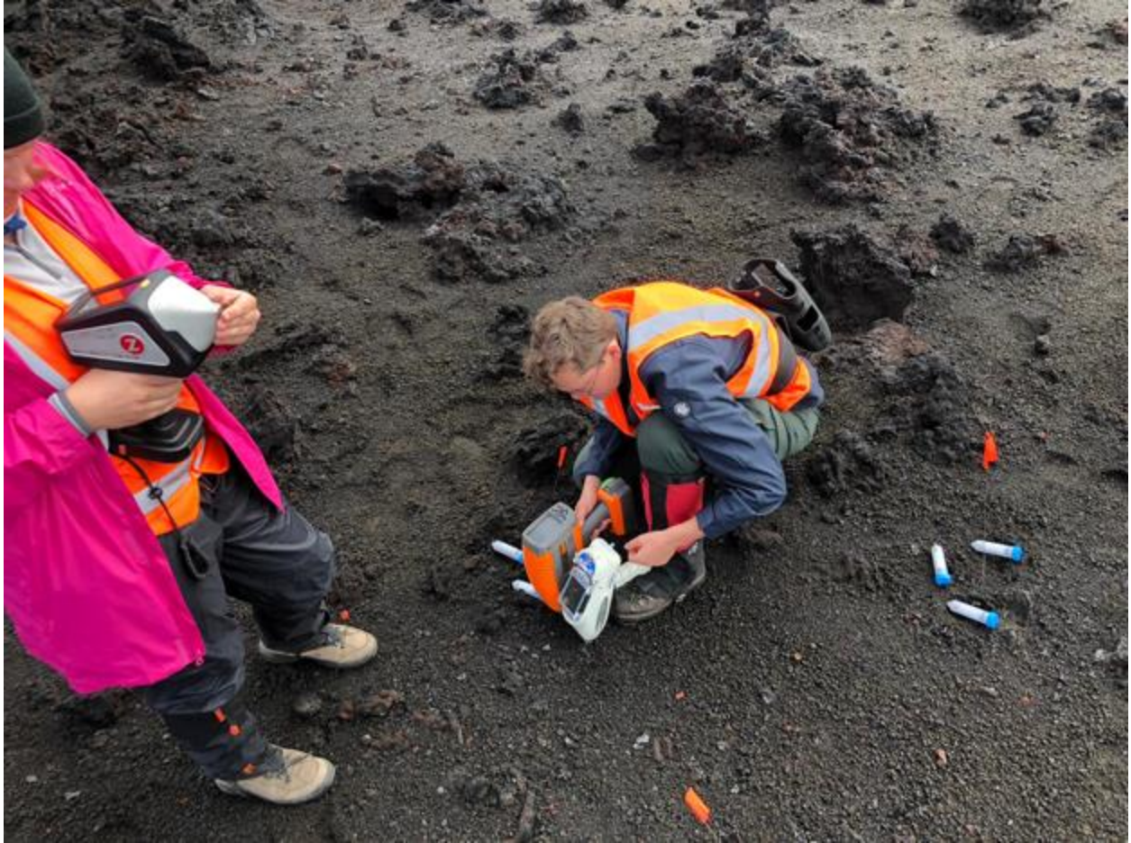
Figure 6: I use the LIBS to measure elemental concentrations of small rocks while Professor Erika Rader of the University of Idaho uses the ASD and XRF to collect X-ray and visible/near IR spectra of the sediment. Photo credit: Carlie Novak
