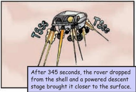
After 345 seconds, the rover dropped from the shell and a powered descent stage brought it closer to the surface.
