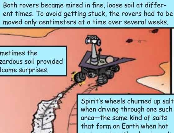
Both rovers became mired in fine, loose soil at different times. To avoid getting stuck, the rovers had to be moved only centimeters at a time over several weeks.
