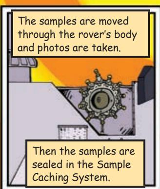
The samples are moved through the rover's body and photos are taken.
