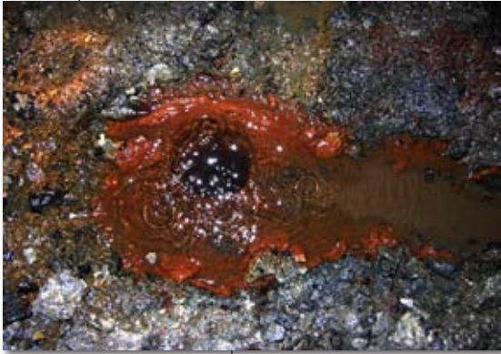
Figure 4.1: Looking down on bubbles of methane gas escaping from a borehole (about 8 mm in diameter) 1130 meters underground in the Lupin gold mine, Nunavut Territories, Canada
