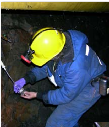
Figure 2.1: Lisa Pratt (Indiana University) backflushing cells on filters to collect biomass samples from deep groundwater in Lupin gold mine, Nunavut Territories, Canada. Note the use of gloves to minimize contamination from hands. Image credit: Lisa M. Pratt
