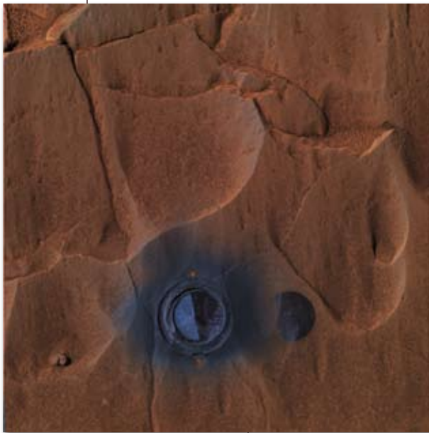
Figure 4.2: This image was taken by the Mars Exploration Rover Spirit's panoramic camera during the rover's grinding of the rock dubbed "Mazatzal" with its rock abrasion tool. The picture shows the rock after the rover drilled 3.8 millimeters (.15 inches) into the target dubbed "New York" on Sol 82. The dark grey coating seen after brushing remains on the right side of the hole, while the left side is the underlying basaltic rock. This approximate true-color image was created using the panoramic camera's red, green and blue filters. Image credit: NASA/JPL/Cornell
