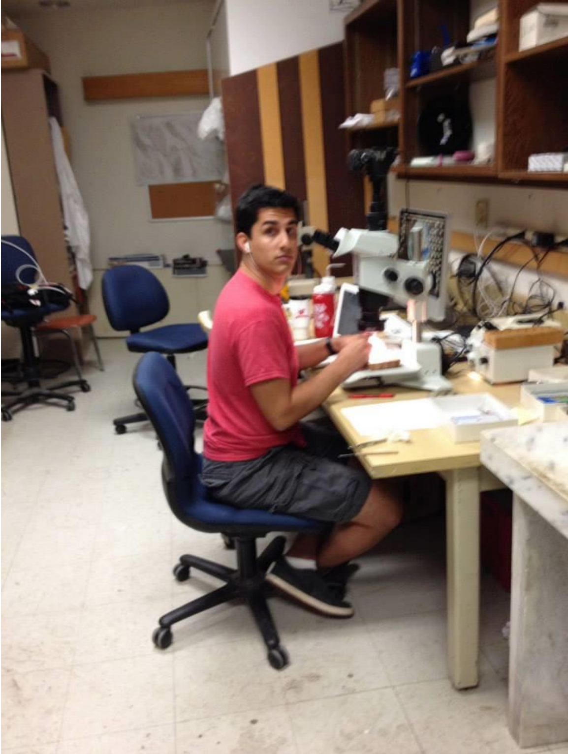
Image 2: Grain picking from a sample. After grain picking, samples are carbon coated and surveyed using a scanning electron microscope (SEM).
