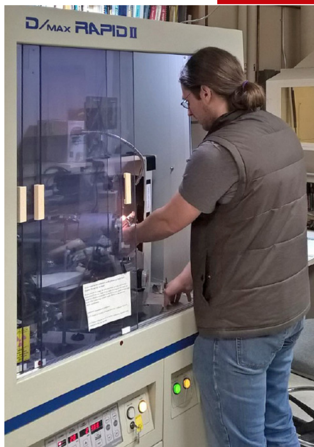
Fig. 1. Graduate student Franklin Hobbs loading a sample of microbial dolomite for XRD analysis. Image credit: Huifang Xu.
