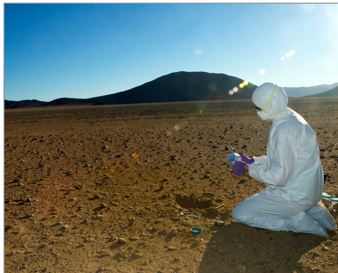
Figure 1: Soil samples being collected by Wilhelm in a clean room suit to minimize introduction of anthropogenic contaminants while sampling in the Atacama Desert (photo credit: A. Davila).
